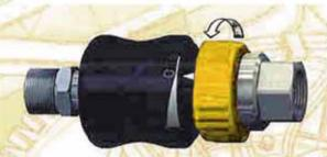
Rotation of the ring from the "Lock" position to Zero (the nipple is blocked)
